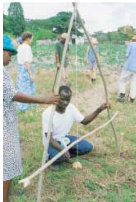
Participants in a PELUM-organised workshop on soil conservation and land-use planning learning how to use an A-frame, a simple device for marking contours on a slope (Photo: PELUM)
